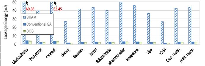
Fig. 7. LLC leakage energy comparison for SRAM, conventional SA, and SOS.
