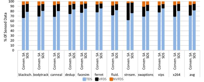
Fig. 8. Distribution of sensed data. SOS is equipped with  $MTJ_{Ref}=4.8K\Omega$ , TMR=150%, and 10% variation in TMR.
