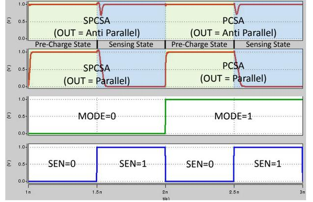
Fig. 4. Transition waveforms of PCSA and SPCSA.
