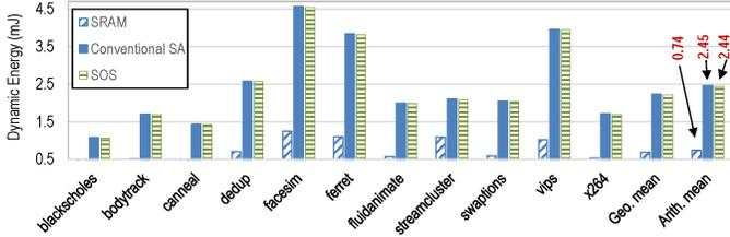
Fig. 6. LLC dynamic energy comparison for SRAM, conventional SA, and SOS.
