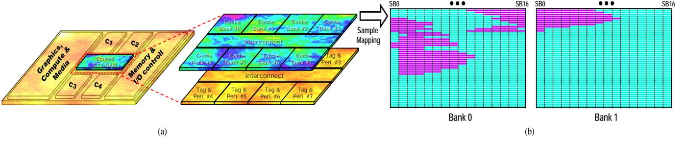
Fig. 2. (a) PV map of a 4-core CMP die, (b) Determining the preferred SA circuit based on post-fabrication sub-bank resiliency assessment to PV.
