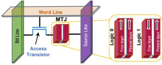
Fig. 1. An illustration of a 1T1R STT-MRAM cell embedded in the cache organization.
