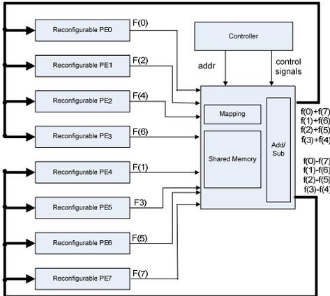
Fig. 2. Top level architecture of scalable DCT
