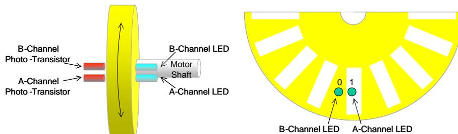
**Fig. 3.** Rotating shaft application for a quadrature decoder.
