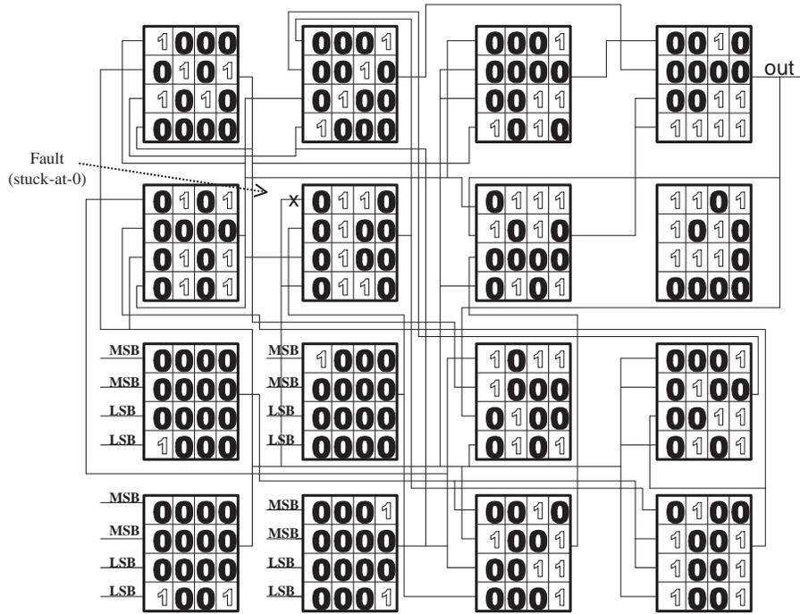
**Fig. 6.** Evolved configuration showing routing, LUT contents, and simulated fault. Inputs are on the lines labeled MSB and LSB, referring to the least/most significant bit of the input. Wires that are shown crossing perpendicularly (eg, +) are unconnected – only wires that have T junctions are connected.
