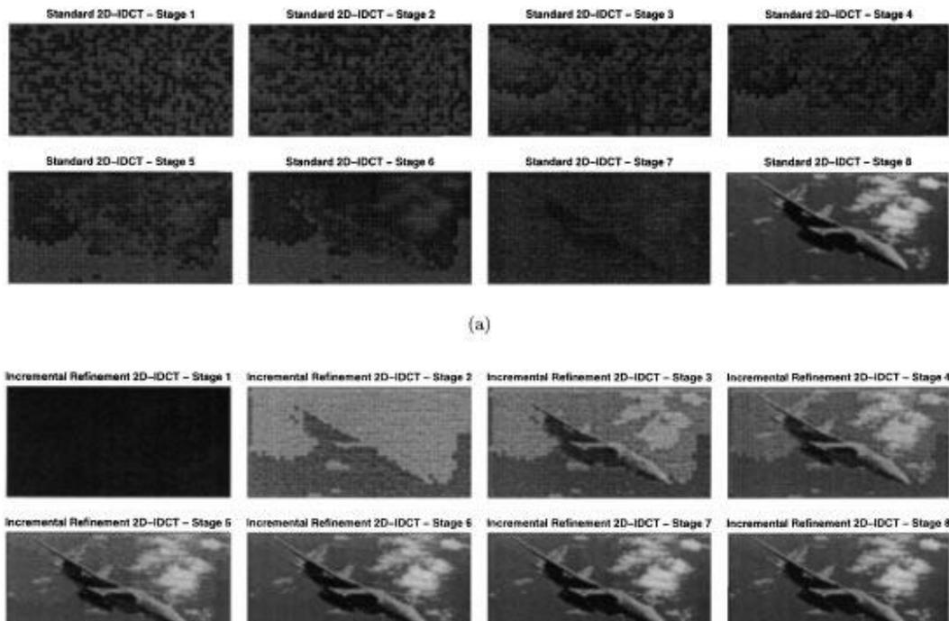
Figure 2. (a) The successive results obtained using a standard distributed arithmetic approach to performing the 2D-IDCT (b) The results obtained during 8 successive stages of 2D-IDCT refinement using the successive refinement architecture described in the text.[1]
