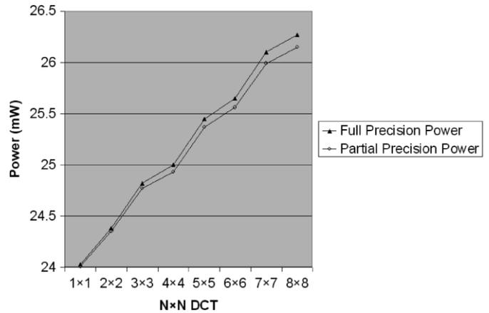
Fig. 3 Comparison of power consumption of different zones of DCT [2]
