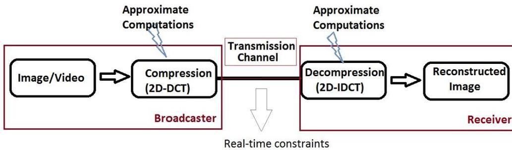
Figure 1. A simplified video broadcaster-receiver scenario showing target of approximate computations
