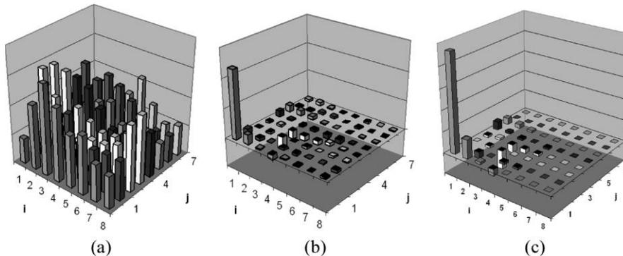
Fig. 4 (a) Normalized 8x8 block of image data. (b) Output of 2-D DCT (64 DCT coefficients). (c) Output of quantization operation
