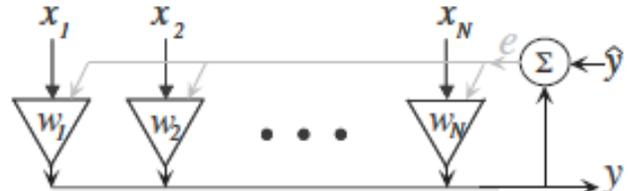
Fig. 8. Utilizing RASP's floating-gate transistors to realize adaptive filters and neural networks [2].
