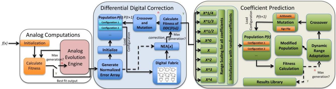
Fig. 2. Schematic of ECHELON technique. The two stages of ECHELON are shown in blue and green colors, receiving analog pre-processed inputs.
