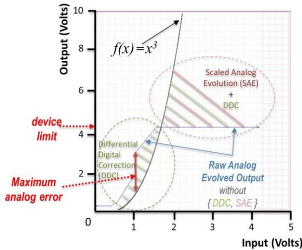
Fig. 3. Example of evolution of cube of independent variable and how analog and digital correction improve accuracy in respective regions of operation [3].
