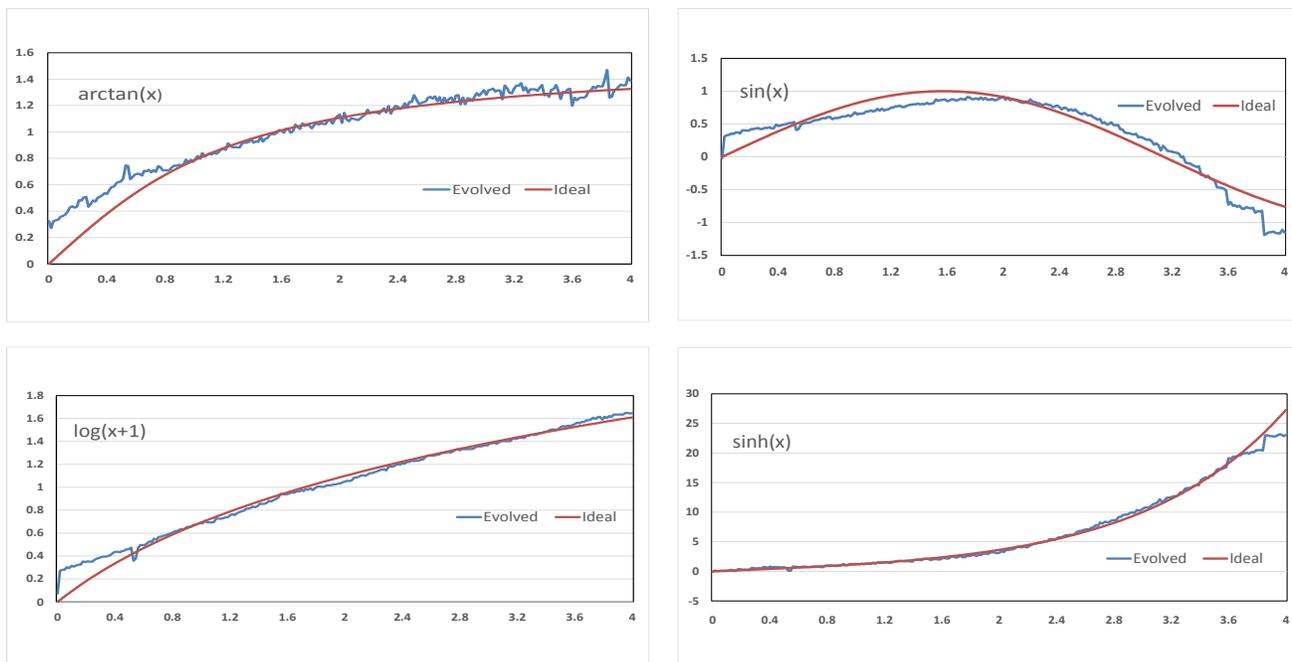
Fig. 9. ECHOLON evolved circuits (blue) approximating  $\arctan(x)$ ,  $\sin(x)$ ,  $\log(1+x)$  and  $\sinh(x)$  as a Puiseux series in  $x^{(1/4)}$ ,  $x^{(1/3)}$ ,  $x^{(1/2)}$ ,  $x^0$ ,  $x$ ,  $x^2$ ,  $x^3$ ,  $x^4/x^{(1/5)}$  or the Pade approximant with the corresponding ideal curves (red) indicating relative performance of ECHOLON
