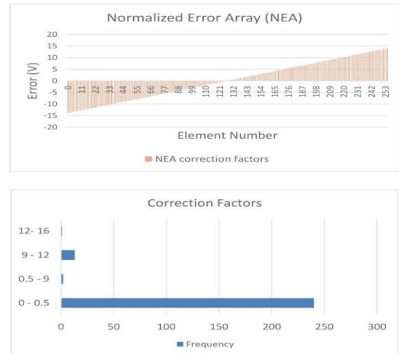
Fig. 4. Elements of the NEA or normalized differences appearing as fractions of the maximum analog error (above) and correction factors evolved (below) for each point on  $x^3$  indexed by  $D[i]$  by DDC.
