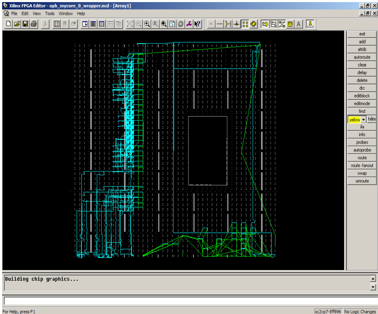
Figure 23: Partial Reconfiguration Module Routing
