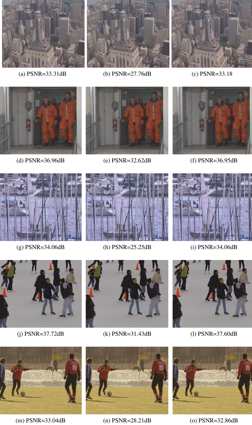
Figure 15: Fault recovery results for various 4cif test video sequences [27] - left: images in frame buffer of 142mW healthy DCT, center: 142mW faulty DCT, right: post fault-recovery 119mW DCT
