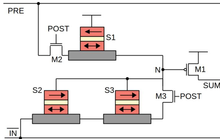
Figure 31: The three-bit hybrid spin-CMOS synapse. © 2019 IEEE.
