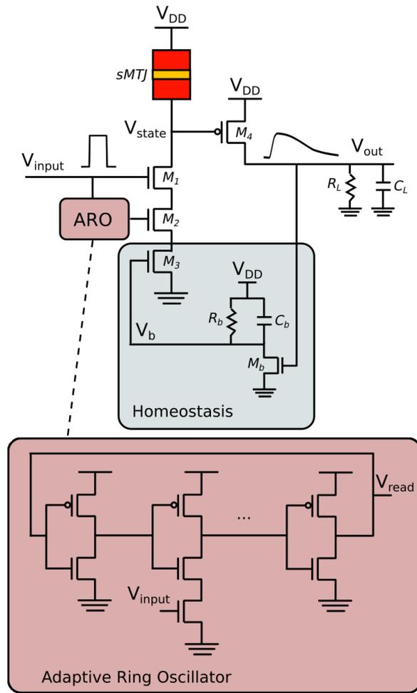
Figure 26: The Subthreshold Spintronic Stochastic Spiking Neuron circuit.
