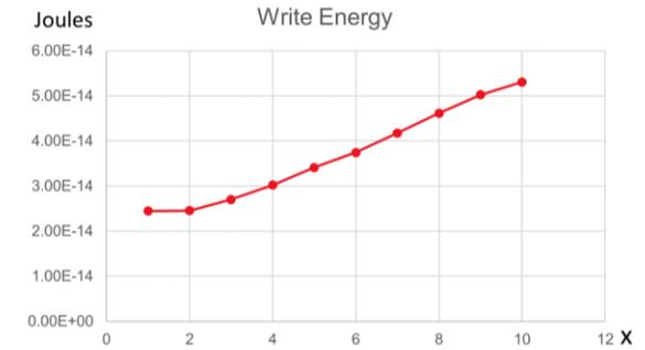
Figure 13: Left side – relation of performance characteristics to TMR. Right side – relation of performance characteristics to driving transistor width (nMOS width =  $Fw$  and pMOS with =  $2Fw$  where  $F$  is the minimum feature size). © 2018 IEEE.
