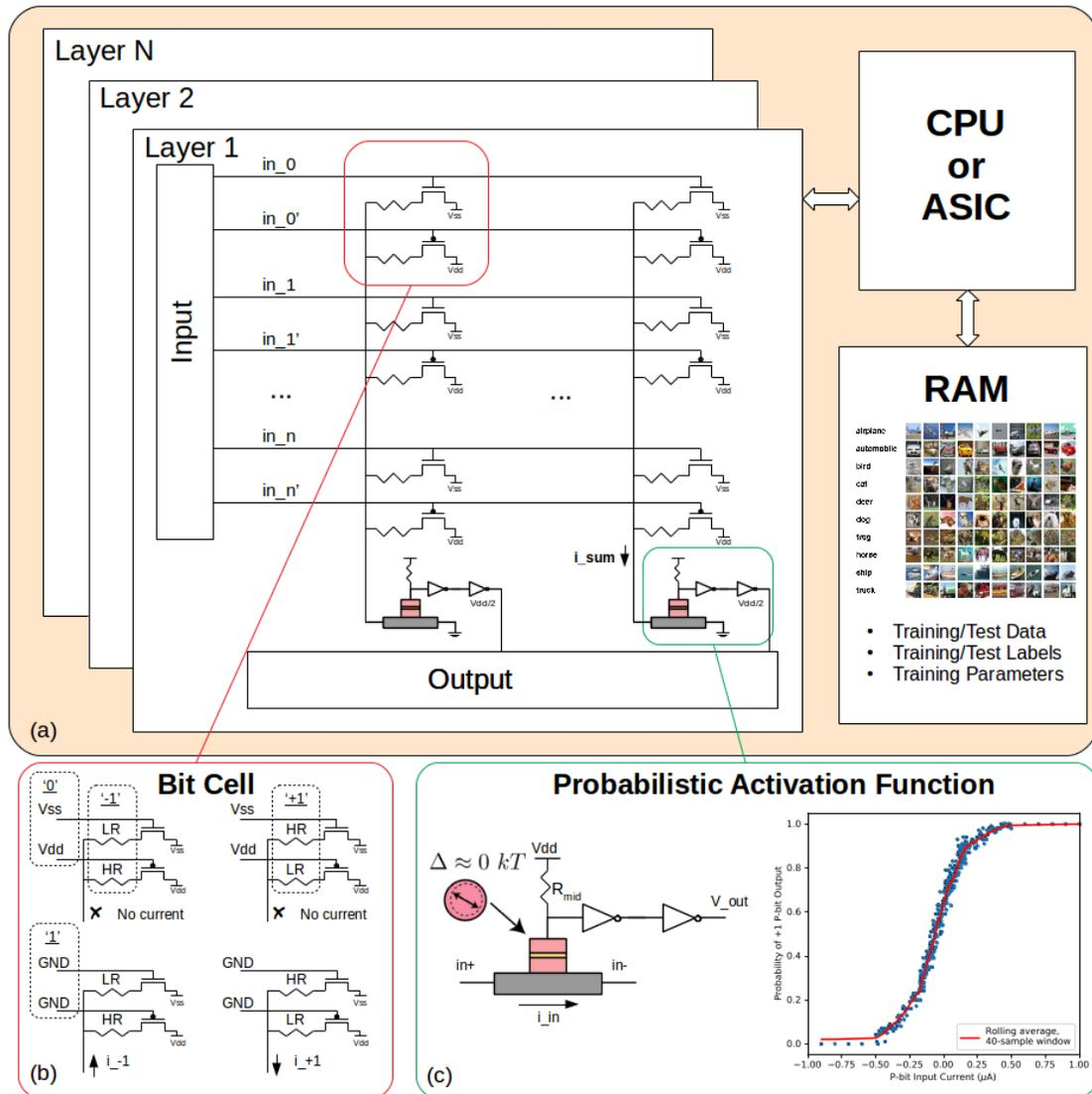
Figure 17: Neuromorphic accelerator proposed in this Chapter. © 2019 IEEE.
