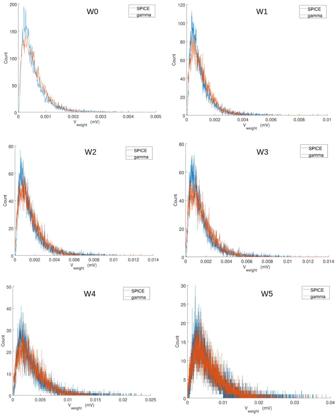
Figure 35: Synapse weight distributions for SPICE simulations and fitted gamma parameters.
