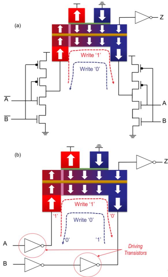
Figure 11: Two Spintronic Muller C-Element Designs. © 2018 IEEE.
