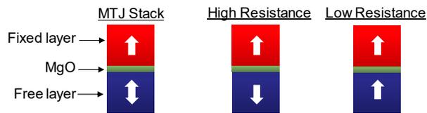
Figure 1: Illustration of the MTJ stack, high resistance state, and low resistance state.
