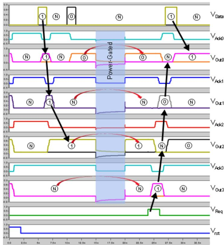
Figure 14: Asynchronous 4-phase dual-rail FIFO pipeline design, performance characteristics, and functional verification showing instant on/off after power gating. © 2018 IEEE.
