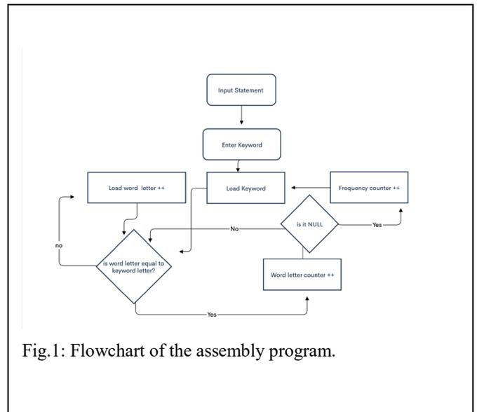
Fig.1: Flowchart of the assembly program.
