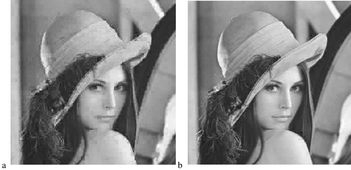
Figure 4.3: CS reconstruction of compressed Lena image partitioned into 10 \times 10 blocks, each sampled using a 40 \times 100 measurement matrix with 200 bits per row allocated a) uniformly and b) adaptively.
